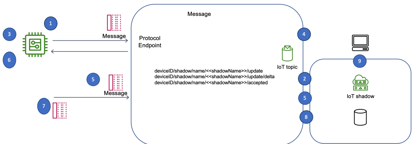
Figure 3: Using AWS IoT Device Shadow service with devices.
