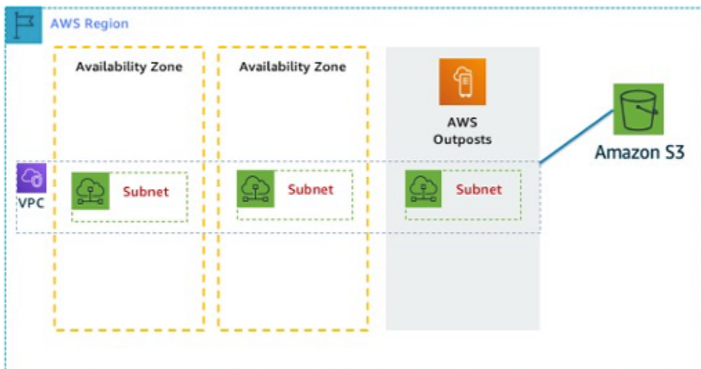
Example AWS Outposts architecture
